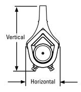
Horizontal Clearance Required Standard Duty: 110 mm (4-1/4") Heavy Duty: 135 mm (5-1/4")
